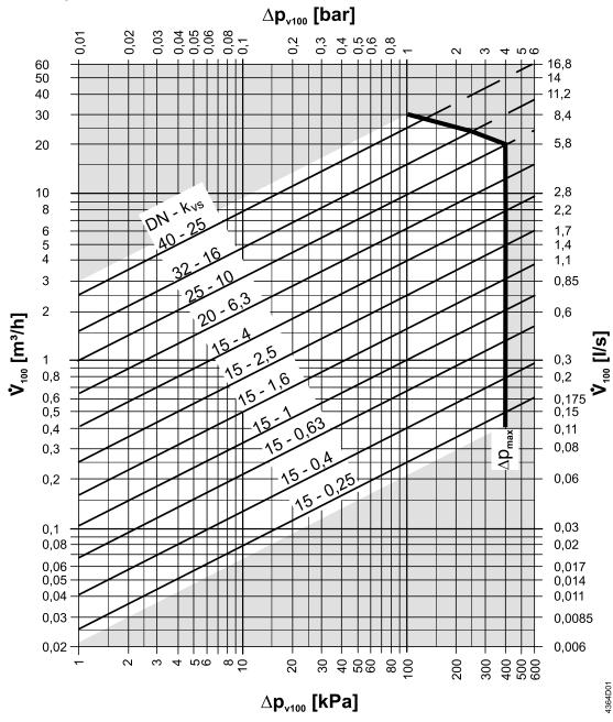
$\Delta p_{\text{max}}$  = Maximum permissible differential pressure across the valve (VXG44..: mixing port: Ports A-AB, B-AB, diverting: Ports AB-A, AB-B), valid for the entire actuating range valve-actuator unit
