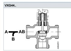
Guided parabolic plug (as of DN25) which is integrated in the valve stem.  $\,$
