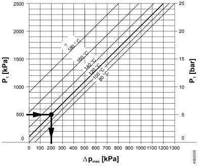
Δp<sub>max</sub> = Differential pressure at a nearly closed valve to largely avoid cavitation
